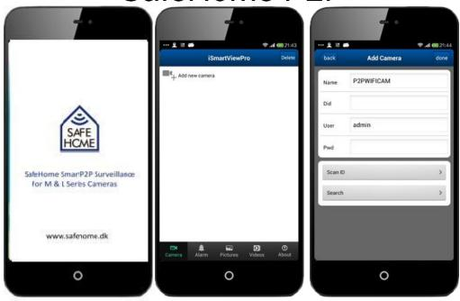
There are three way to add device, that is add manually, scan ID to add and search in LAN to add. ☆ Scan ID and search in LAN to Add as below.
